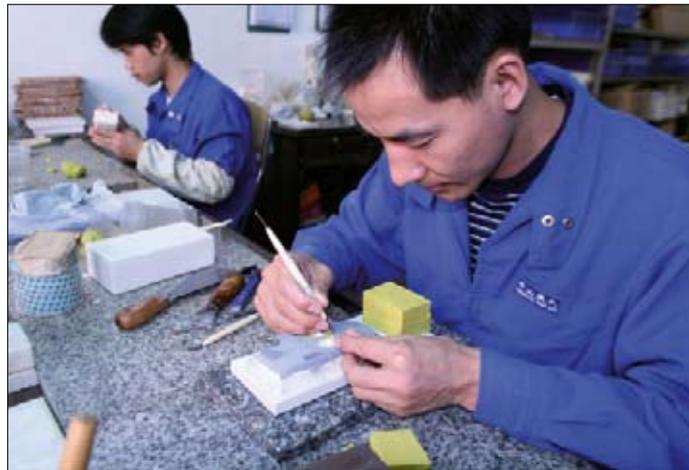
**above and below** Craftsmen all working on hand carving the original masters from which Spark produces its moulds. The girl seen bottom right is working on detail pre-paint finishing of resin cast bodies, which occasionally require filling and fine sanding, while he second girl (immediately below) works in assembly and is applying waterslide decals which Spark use in combination with pad printing to finish its models.
